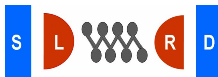
FIG. 1. (Color online) Schematic of the considered system including large electron reservoirs labeled as S and D , respectively, metal nanoclusters L and R , and the molecule placed in between.
